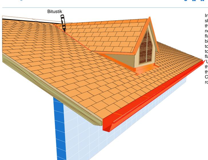
Install the bituminous shingles on the dormer up to the center of the valley. Do not nail shingles on the valley flashing but use a line of bitustick on each shingle raw to glue shingles together and to glue them on the valley flashing.
