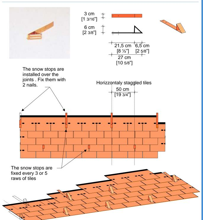
The drawing shows the position of snow stops every 3 raws of tiles, to obtain a density of snow stops of 2,33 pieces every m² (25 sq.).
